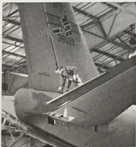
Tech. Sgt. Brandon Matthews works a corrosion measure on one of the unit's KC-135R aircraft.
